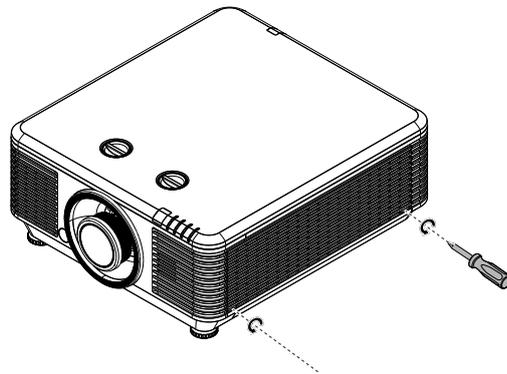
2. Remove the filter module from the projector
