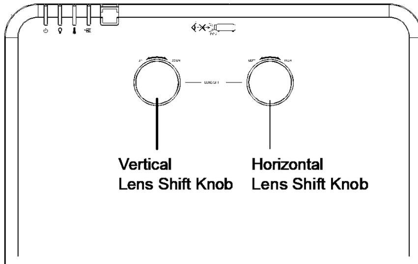
The Lens Shift feature provides a lens shift function that can be used to adjust the position of the projected image either horizontally or vertically within the range detailed below.
