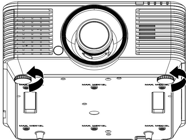
2. To lower the level of the projector, lift the projector and twist the adjusters clockwise.
