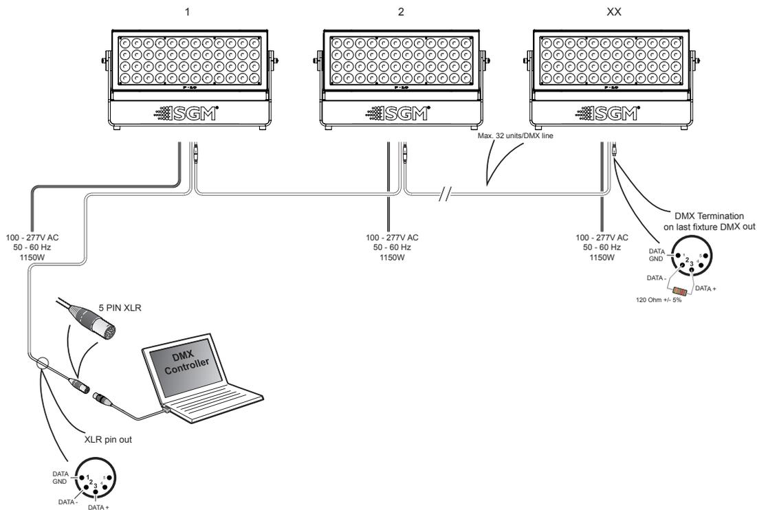
Figure 11: P-10 connection diagram (see page 17 for POI)
