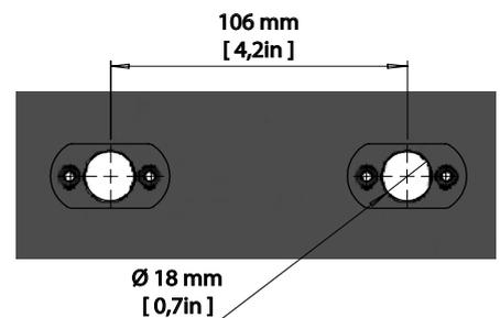
Figure 2: P-10 Series locking points
